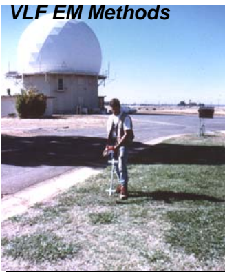
Metrotech Utility Locator
