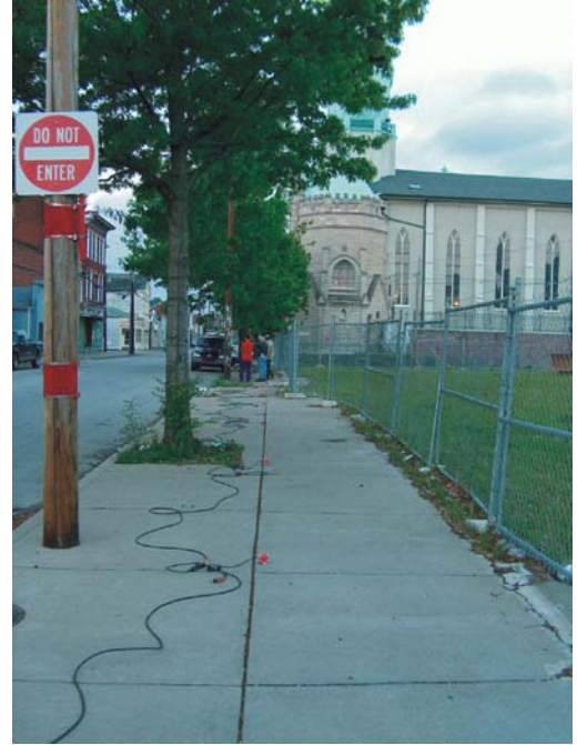
Microtremor Measurements along Sidewalk
