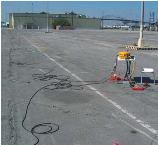
Refraction Microtremor Array Layout
